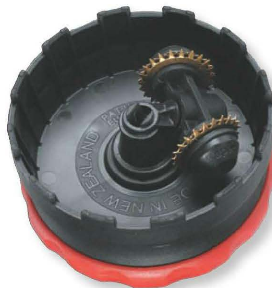
A wallpaper scorer perforates the waterproof coating so wallpaper stripping solution can penetrate into the glue layer between the wallpaper and the wall.
