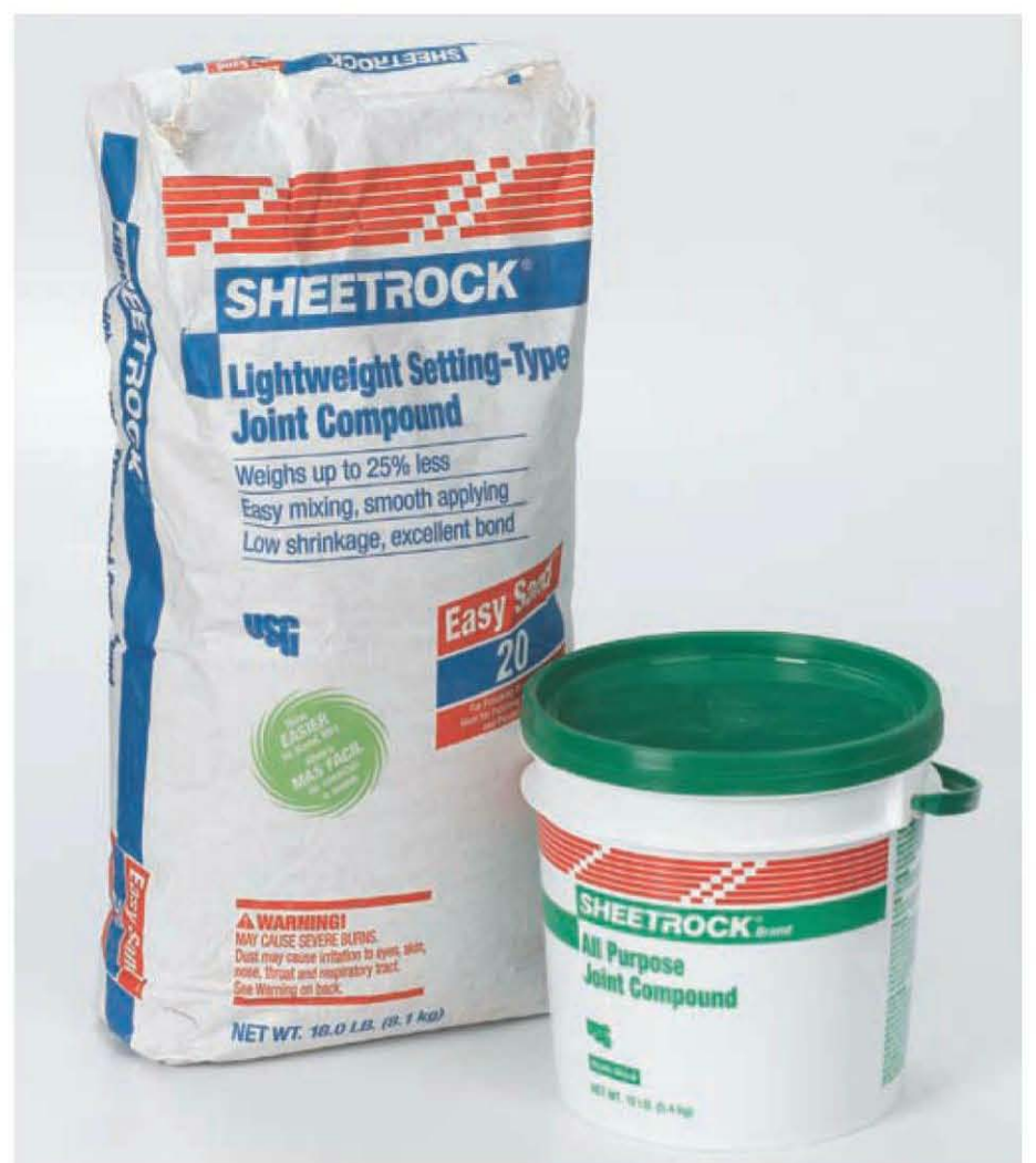
Premixed joint compound (right) is convenient, but it tends to shrink and crack and the shelf-life isn't very long once the tub is opened. Dry bagged joint compound (left) can be mixed with water in small batches, dries smoothly, and comes in a wider range of types with special application and drying characteristics.
