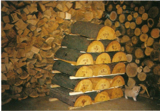
Figure 8.9 • End-coated half-log sections of eastern white pine are stickered and open-piled for slow drying. (Photo by R. Bruce Hoadley)
