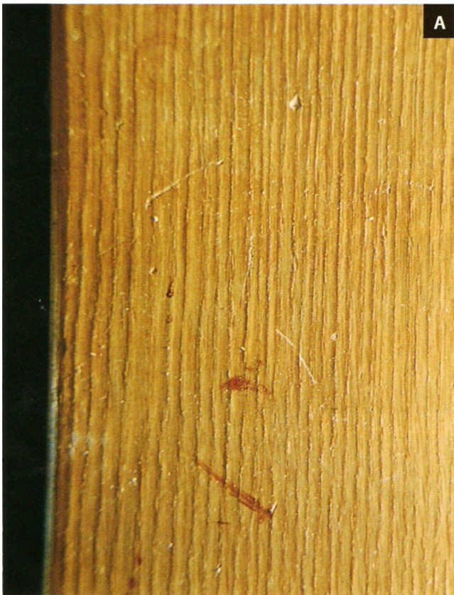
Figure 14.7 • After several years of exposure to variable humidity, the lathe checks in the oak veneer on this cabinet fractured the surface coating of varnish (A). The corrugation on this maple veneer identifies the loose surface (B). (Photo A by R. Bruce Hoadley; photo B by Richard Starr)
