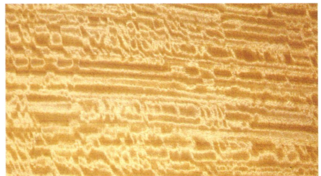
Figure 2.16 • Broken-stripe figure in Ceylon satinwood, sometimes referred to as bee's-wing figure. (Photo by R. Bruce Hoadley)
