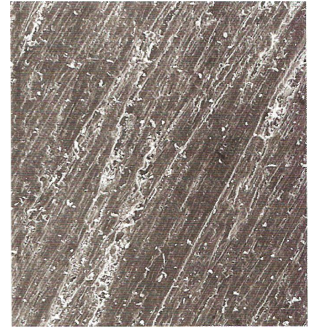
Figure 12.4 • The sample sanded with 220-grit paper looks much like the scraped surface, although there are more visible scratches. Dust, rather than torn fibers, seems to have filled the open vessels. A surface like this would feel quite smooth to the touch. 50X magnification. (Photo by Stephen Smulski)
