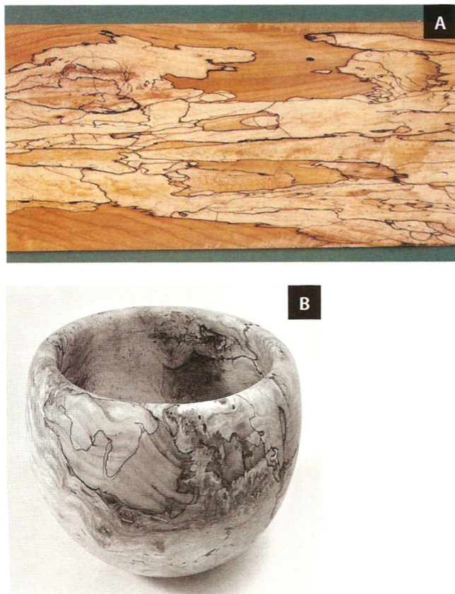
Figure 2.47 • As certain white rots develop, dark zone lines form, as on this piece of sugar maple (A). This type of decay is called spalting. The turned bowl of spalped maple was made by Mark Lindquist (B). (Photo A by Randy O'Rourke; photo B by Richard Starr)
