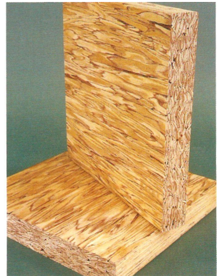
Figure 16.8 • Parallel strand lumber (PSL) utilizes materials unusable for making LVL. Though of uniform strength and reliability, PSL is relatively heavy and has a rough, porous surface. This example shows the random arrangement of aligned veneer strands. (Photo by Randy O'Rourke)
