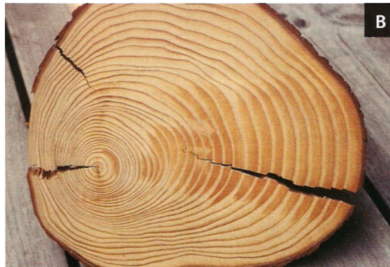
Figure 2.35 • Wide growth rings surrounding the pith (left) are juvenile wood, which is lighter and weaker than narrow-ringed mature wood. In the photo on the right, needle scars appearing as dots on the wood also indicate juvenile wood. (Photos by Randy O'Rourke)
