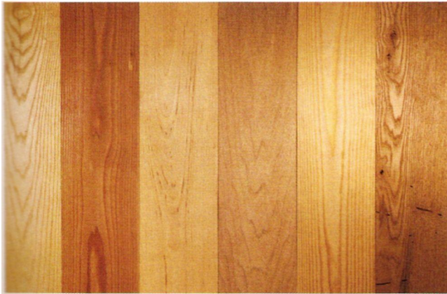
Figure 2.6 • FLATSAWN FIGURE IS CHARACTERIZED BY OVAL, U-SHAPED, and V-SHAPED PATTERNS. BOARDS (LEFT TO RIGHT) ARE ASH, CHERRY, SOUTHERN YELLOW PINE, CHESTNUT, WHITE BIRCH, AND EASTERN SPRUCE. PHOTO BY R. BRUCE HOADLEY)
