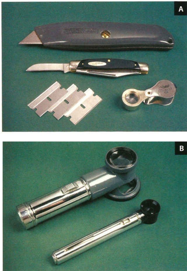
Figure 3.5 •Tools for macroscopic identification are few and simple: a 10x hand lens and a means of cutting wood surfaces cleanly. A very sharp knife or an industrial single-edged razor blade is satisfactory (A). Some lenses have built-in lights (B). (Photos by Randy O'Rourke)
