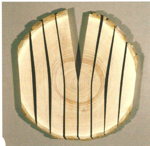
Figure 6.16 • The severity of cupping in a board is related to its position in the log. (Photo by R. Bruce Hoadley)
