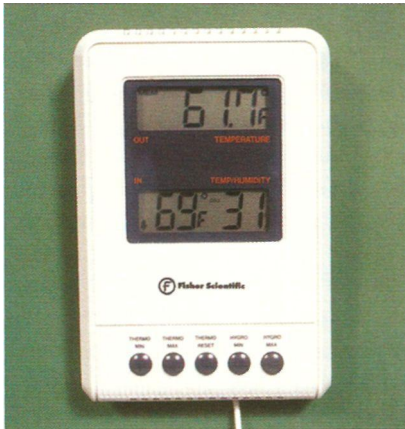
Figure 7.12 • A digital hygrometer usually comes with a thermometer. Easy to read and handy, its only drawback is that there is a lag time of several minutes when the humidity level changes. (Photo by Randy O'Rourke)
