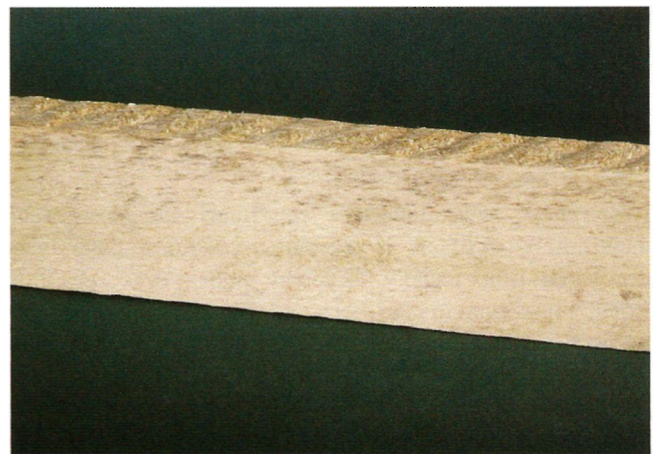
Figure 2.42 • The abnormal fibers of tension wood can leave a woolly surface, as on this cottonwood board when it was sawn from the log. (Photo by Randy O'Rourke)
