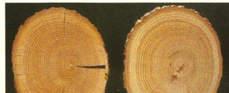
No treatment; disk with checks. 50% solution, 1 day at 140°F; disk without checks.
