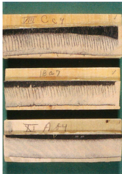
Figure 14.8 • To indicate the depth of lathe checks, strips of veneer are brushed under dye, glued to blocks, and then leveled on a disk sander. (Photo by Randy O'Rourke)
