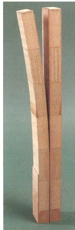
Figure 7.4 • The consequences of unbalanced construction are evident here, where crossband and face veneer have been bandsawn off one side of a strip of lumber-core panel. (Photo by Randy O'Rourke)
