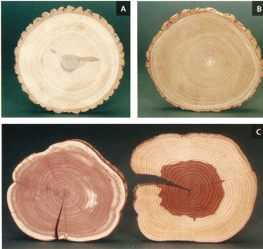
Figure 1.10 • The relative width of the sapwood varies according to species; heartwood (dark area) is small in white ash (A) and wide in catalpa (B). Heartwood/sapwood growth may also vary tremendously within a species, according to growing conditions. Both discs (C) were cut from eastern redcedar trees. The sample on the left was shaded by the larger trees around it reducing its crown. The one on the right grew normally in an open meadow with a full crown of foliage and greater need for sap conduction. (Photos by Randy O'Rourke)
