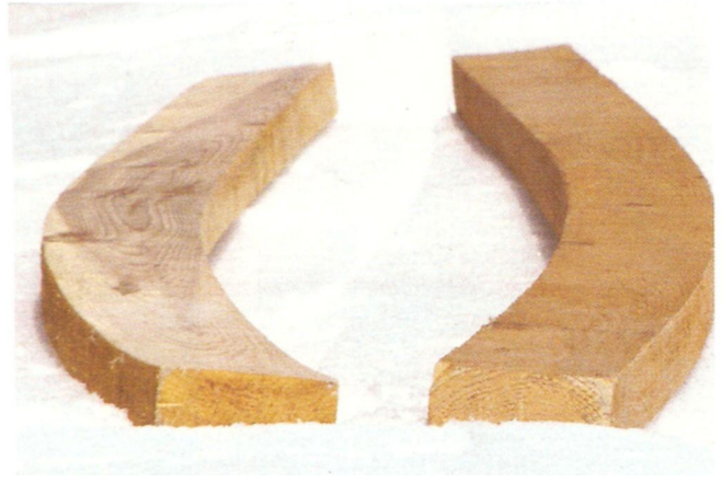
Figure 2.39 • Severe crook in roughsawn lumber caused by compression wood. (Photo by R. Bruce Hoadley)
