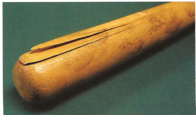
Figure 4.10 • Hitting a baseball on the tangential surface of this white ash bat has caused "chipping" or separation of the growth layers by compression failure in the weaker earlywood. (Photo by Randy O'Rourke)
