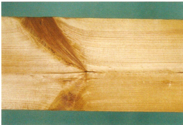
Figure 2.30 • These spike knots show the origin of limbs at the pith. (Photo by Randy O'Rourke)
