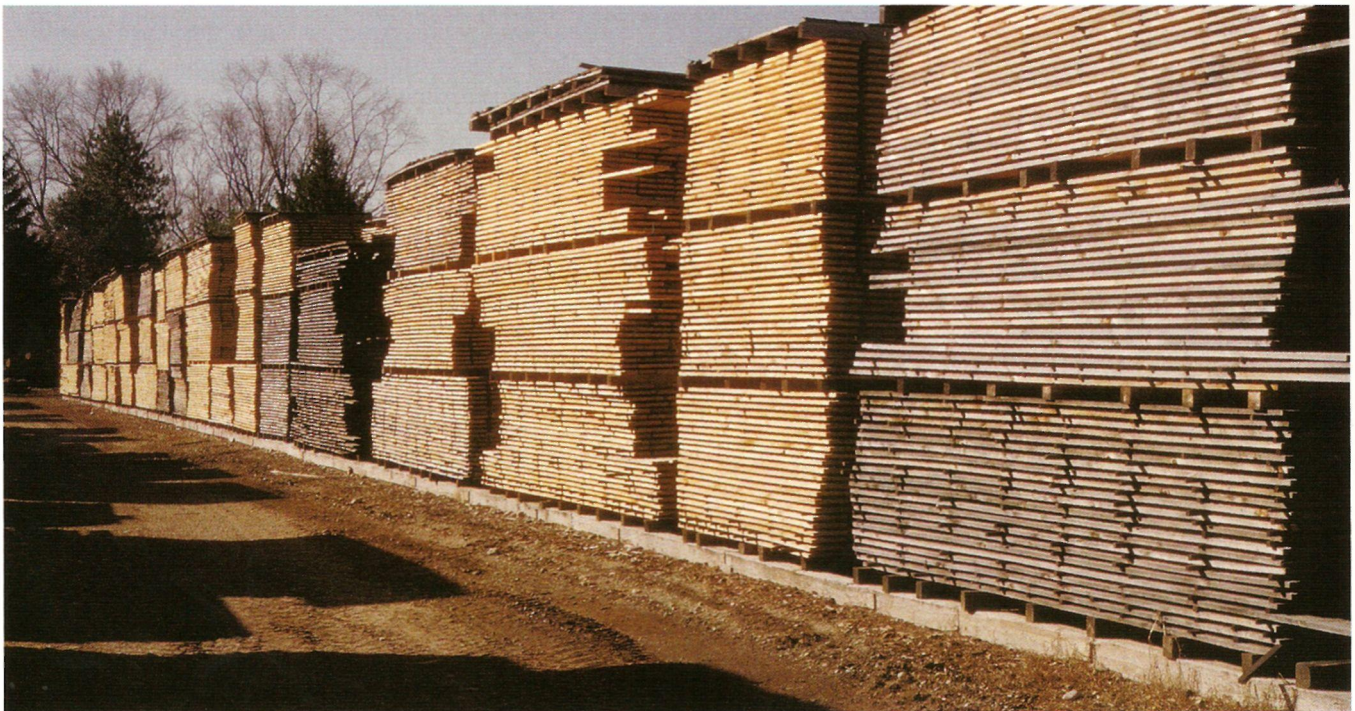
Figure 17.5 • This pine lumber is air-drying at a small, family-owned mill yard, where small orders can be filled at a reasonable price. (Photo by R. Bruce Hoadley)
