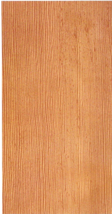
Figure 2.3 • Quarter-sawn surfaces of uneven-grained conifers such as this Douglas-fir board have parallel-grain figure. (Photo by Randy O'Rourke)
