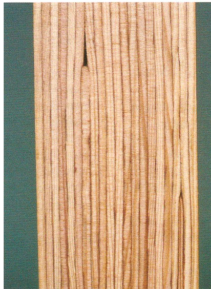
Figure 16.7 • In the manufacture of LVL, weak end-grain butt joints are avoided by overlapping consecutive veneers in a given layer to provide side-grain bonding. (Photo by Randy O'Rourke)
