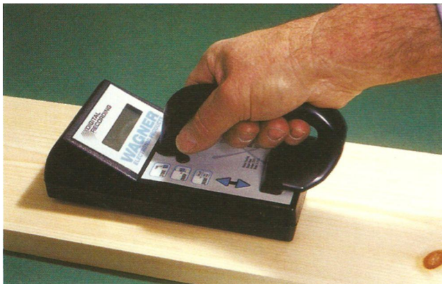
Figure 7.14* The electrode on the back of a dielectric meter generates a radio-frequency field as it is pressed against the face of a board. (Photo by Randy O'Rourke)
