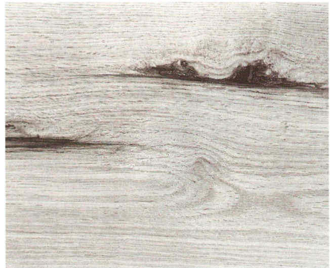
Figure 2.34 • Included bark adjacent to a knot in red oak. This defect may also result from an injury to the growing tree. (Photo by Richard Starr)
