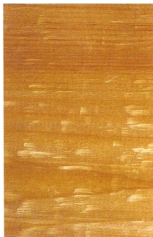
Figure 9.19 • Chip marks are the result when a machine's exhaust system isn't capable of clearing debris from the cutterhead. (Photo by Randy O'Rourke)
