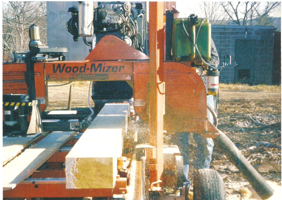
Figure 17.3 • The Wood-Mizer portable mill utilizes a horizontal bandsaw that travels parallel to the log and produces smooth, accurate cuts. (Photo by R. Bruce Hoadley)
