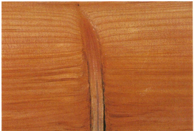
Figure 2.28 • A spike knot showing an intergrown portion (top) and an encased portion (bottom). (Photo by Randy O'Rourke)
