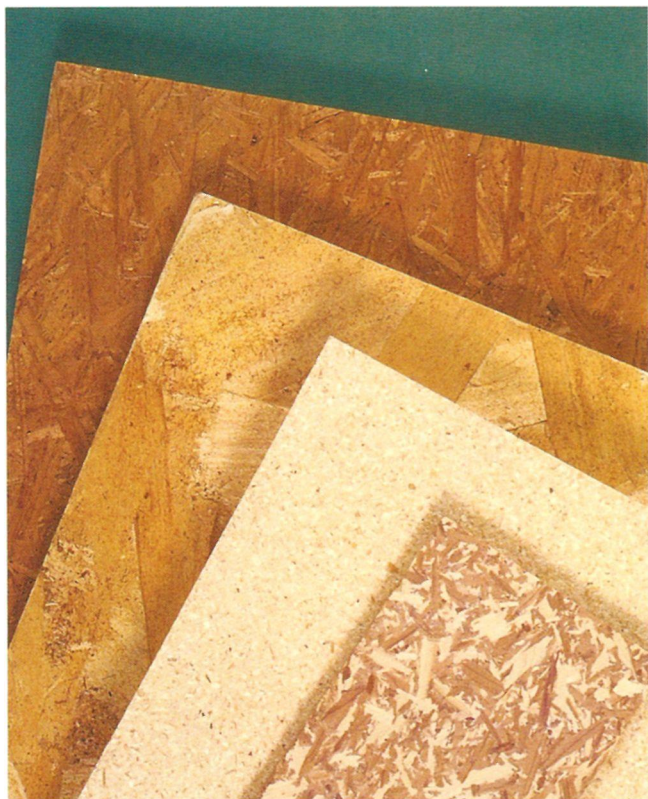
Figure 15.2 • An array of composite panel materials includes (top to bottom) oriented strandboard, structural waferboard, counter-top-grade particleboard, and chipboard cedar-closet liner. (Photo by Randy O'Rourke)
