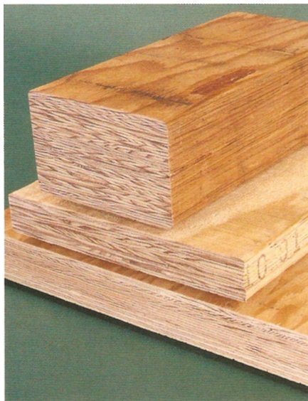
Figure 16.6 • Laminated veneer lumber (LVL) is more consistent in quality than standard lumber, is available in longer lengths, and has a higher stress rating. Here are three examples of LVL. The center piece is a scaffold plank with rough surfaces. (Photo by Randy O'Rourke)
