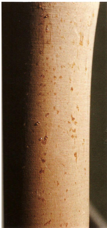
Figure 1.20 • Unless resins are solidified or set by high temperatures in kiln-drying, droplets of resin may exude from the canals as on the surface of this turned baluster of eastern white pine. Resin droplets remain sticky for some time but then harden. Careful scraping or sanding will remove them. (Photo by R. Bruce Hoadley)
