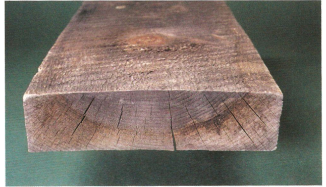
Figure 6.29 • Because drying is more rapid along the grain than across, boards dry first near the ends. The ends shrink before the rest of the board and end checks result. (Photo by Randy O'Rourke)
