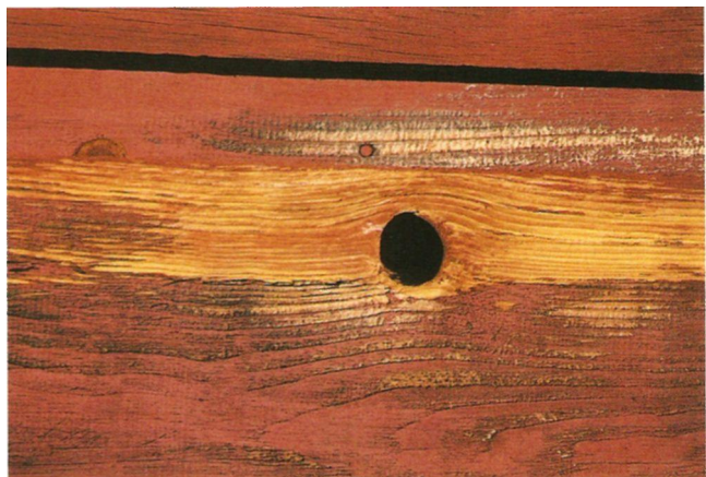
Figure 2.29 • A knothole results when an encased loose knot falls out. (Photo by Randy O'Rourke)
