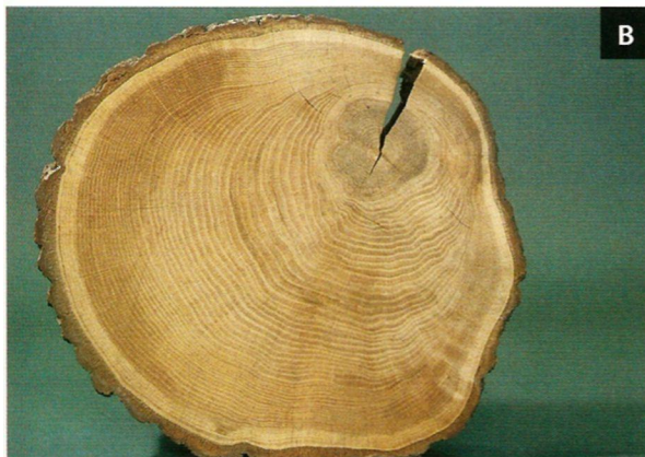
Figure 2.41 • In hardwoods, the reaction wood is on the upper side of the sweep in the tree and is called tension wood. Tension wood looks silvery (A) as shown in the left section after smooth sanding. Tension wood may result in eccentric growth rings in trees (B, C). (Photos A and B by Randy O'Rourke; photo C by Richard Starr)
