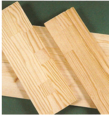
Figure 16.3 • Short pieces of pine are finger-jointed into strips, which are then edge-glued to form wider lumber or panels. These products are sold as "Blockboard" or "Laminate." (Photo by Randy O'Rourke)
