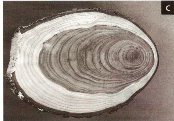
Figure 2.41 • In hardwoods, the reaction wood is on the upper side of the sweep in the tree and is called tension wood. Tension wood looks silvery (A) as shown in the left section after smooth sanding. Tension wood may result in eccentric growth rings in trees (B, C). (Photos A and B by Randy O'Rourke; photo C by Richard Starr)
