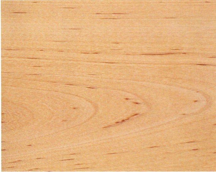
Figure 2.49 • Pith flecks on the tangential surface of this paper birch plank were formed by larvae of tiny flies that burrowed down the tree stem along the cambial layer. (Photo by Randy O'Rourke)
