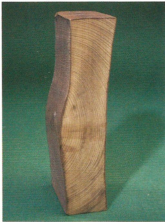
Figure 8.3 • Extreme compression stress in drying may cause wood cells in the core to buckle or collapse, as in this imbuya board, which was sawn rectangular. (Photo by Randy O'Rourke)
