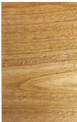
Figure 9.18 • Woolly grain occurs when planing material with a high moisture content or when machining tension wood in hardwoods. (Photo by Randy O'Rourke)
