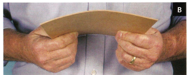
Figure 14.5 • Veneer flexes more easily when checks are opened (A) than when they are closed (B). This simple test distinguishes the tight and loose faces. (Photos by Randy O'Rourke)
