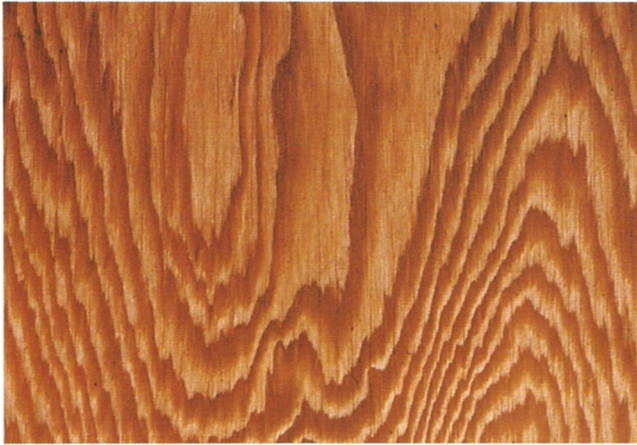
Figure 2.8 • The continuous tangential figure of Douglas-fir plywood is typical of rotary-cut veneer. (Photo by Randy O'Rourke)
