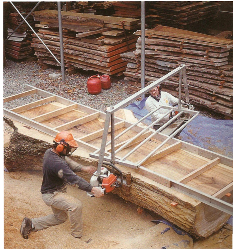
Figure 17.2 • The chain saw mill produces boards from a log. (Photo by Vincent Laurence)
