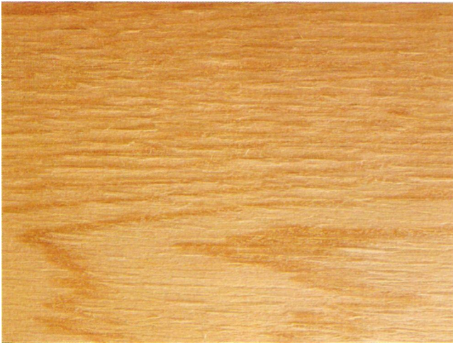
Figure 14.6 • The loose side of Douglas fir veneer shows roughness associated with lathe checks. (Photo by Randy O'Rourke)
