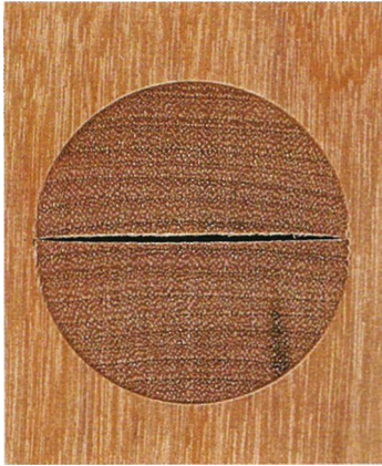
Figure 10.9 • This round tenon was split radially and tangentially before assembly. After moisture cycling, compression shrinkage developed entirely in one direction, opening the radial split. The tangential split remains tightly closed and the glueline is intact. (Photo by Randy O'Rourke)
