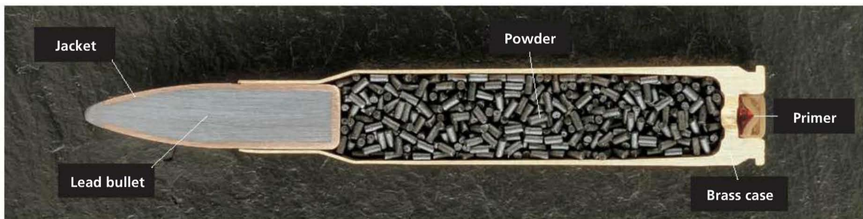
Center-fire cartridges (far left and below) consist of: a brass case; a primer containing a highly explosive compound that ignites when struck by the firing pin; powder, which is ignited by the priming compound; a lead bullet, which may have a copper-zinc jacket to control the bullet's expansion. With rimfires (near left), the firing pin strikes the edge of the rim, igniting the priming compound.
