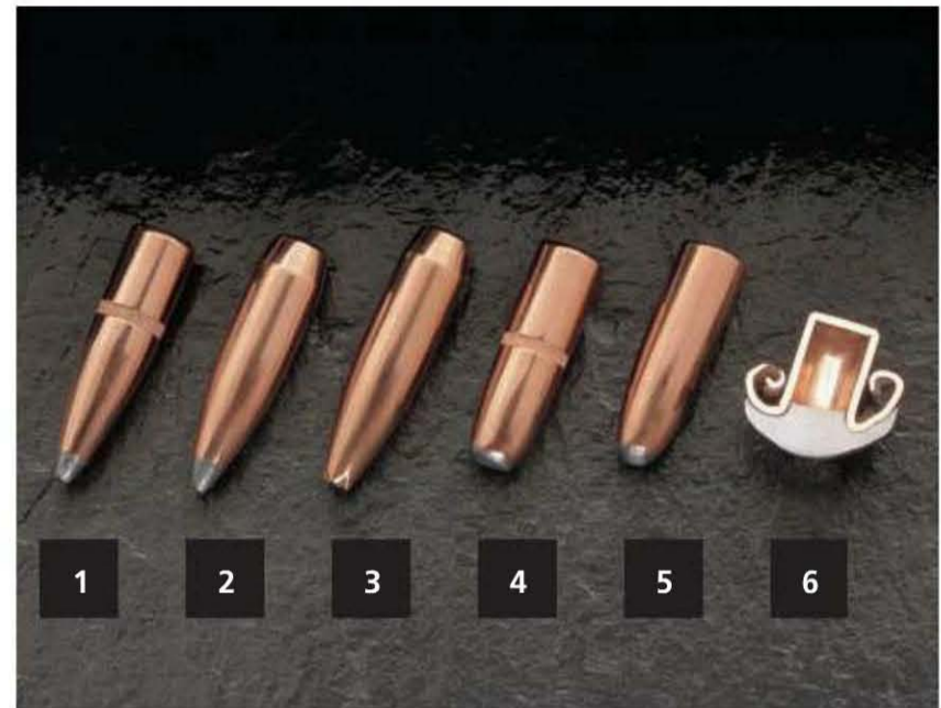
Bullet styles include (1) pointed, streamlined for high velocity and flat trajectory. (2) Pointed boat tail has a tapered base to reduce drag even more. (3) Hollow points mushroom rapidly, but no faster than (4) flat and (5) round points, often used in rifles with tubular magazines. Their blunt points do not detonate cartridges ahead of them, but result in relatively slow flight and short range. (6) Mushroomed bullet shows expansion.
