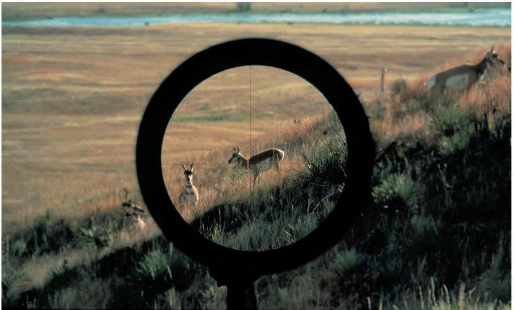
Crosshair reticles work best for long-range shooting. The fine wires provide a precise aiming point and cover little of the target. But the wires may be difficult to see in dim light.
