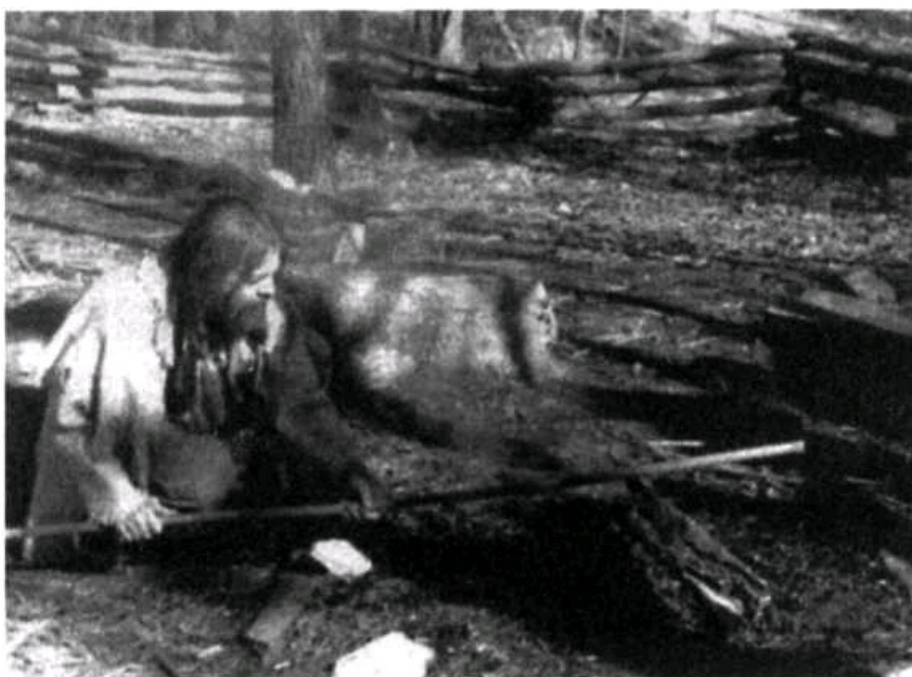
The author heat .straightening the blowgun blank. Bends both at and between the joints must be straightened before interior work begirr.s. (Photo: Michael Eldredge)
