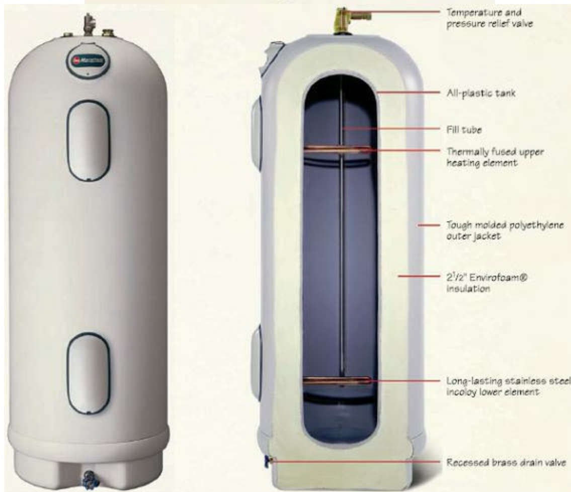
Figure 6.23 Marathon water heater from RUUD and cutaway details.
