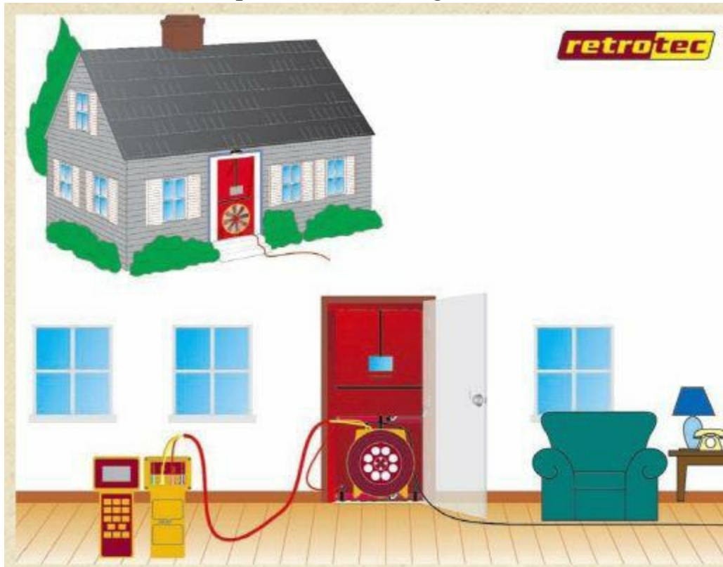
Figure 6.27 Home system with door testing. Illustration courtesy of Retrotec.
