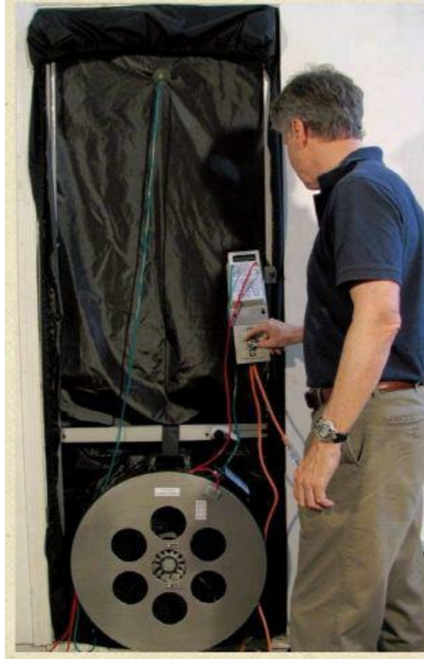
Figure 6.26 Blower door test in process. Photo courtesy of Infiltec Corp.
