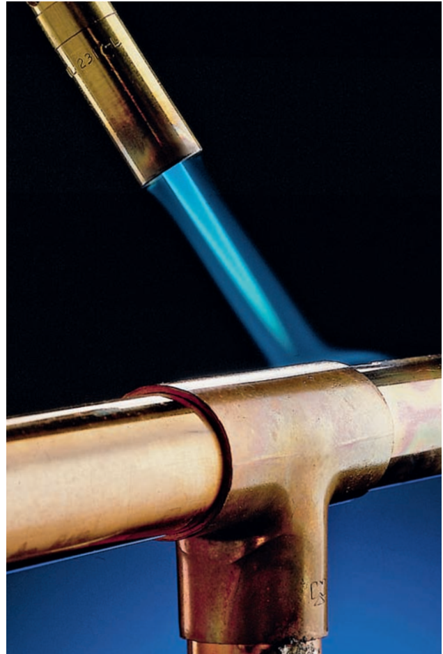
Soldered fittings , also called sweat fittings, often are used to join copper pipes. Correctly soldered fittings (pages 278 to 280) are strong and trouble-free. Copper pipe can also be joined with compression fittings (pages 314 to 315) or flare fittings (page 316). See chart below.
