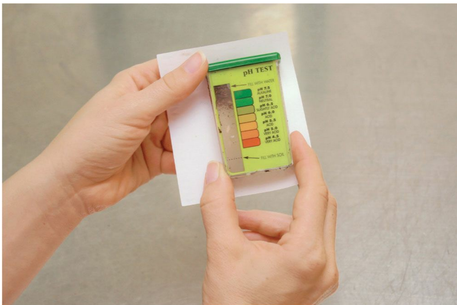
A soil pH test kit is essential for determining how acidic or alkaline your soil is.
