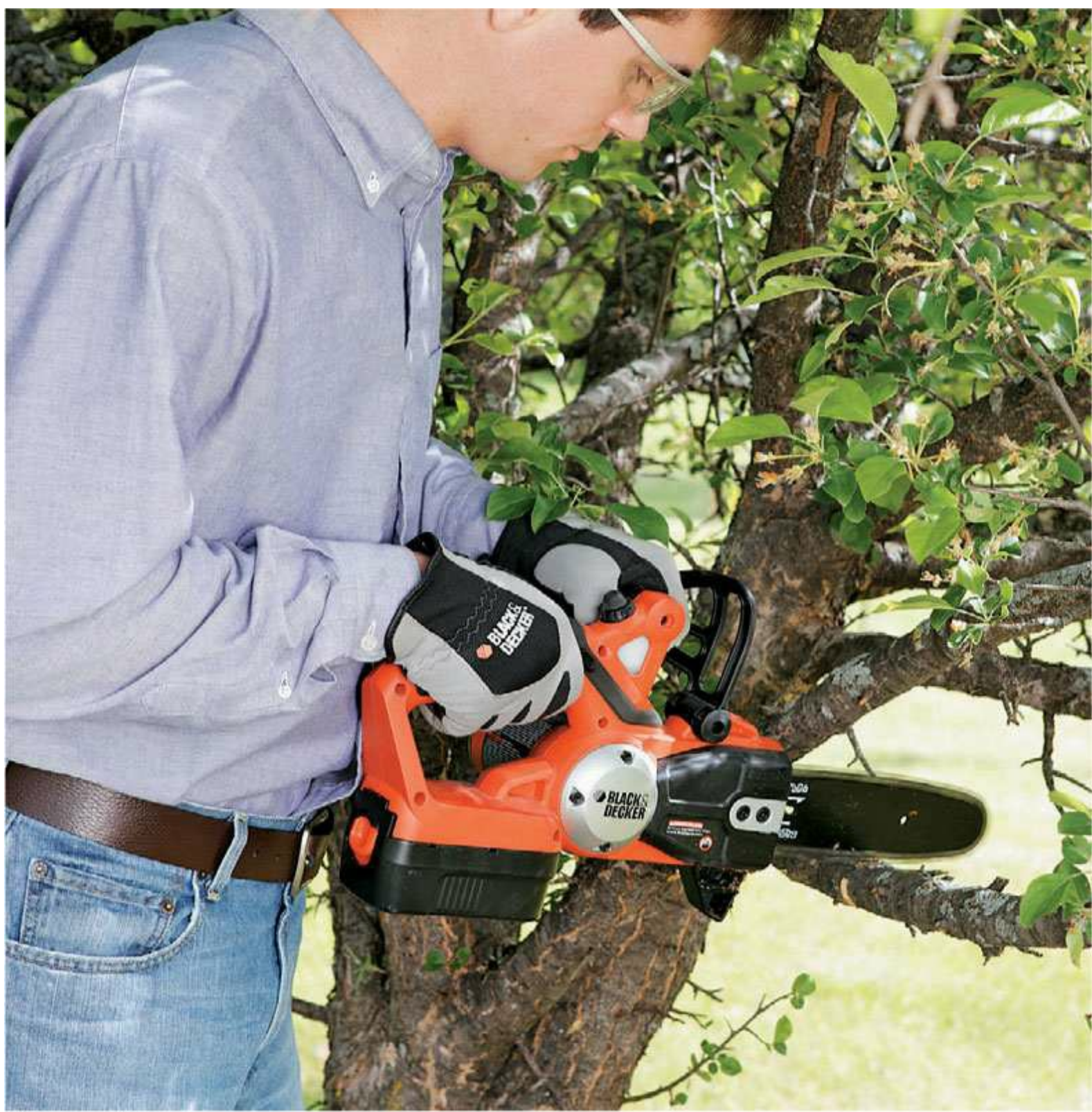
Finish the cut from above. This keeps the bark from tearing when the limb breaks loose.
