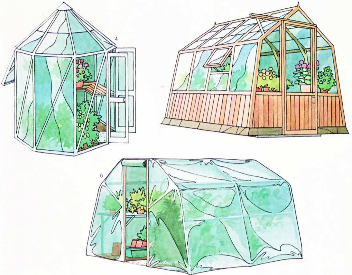
Above Drawings show typical forms and materials of modern greenhouses: 1 Straight-sided alloy-framed; 2 Sloping-sided alloy-framed; 3 Alloy-framed lean-to; 4 Polygonal alloy-framed; 5 Partly boarded cedar-framed; 6 Polythene-covered steel-framed. Far left Permanent benching needs to be sturdily constructed to take the considerable weight of a pot-plant display. Near left Cucumbers (cordon-trained) growing in raised beds of well-rotted compost. The partly boarded sides of the greenhouse reduce heat loss.
