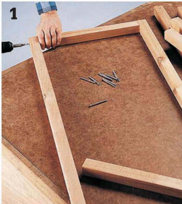
1 Fasten the cleats between the rails to construct the panel frames.
