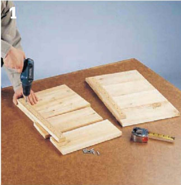
1 Attach the side cleats flush with the tops of the side boards.
