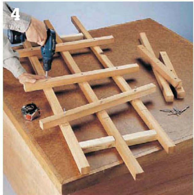
4 Temporary spacers hold the posts in position while the rails are attached.
