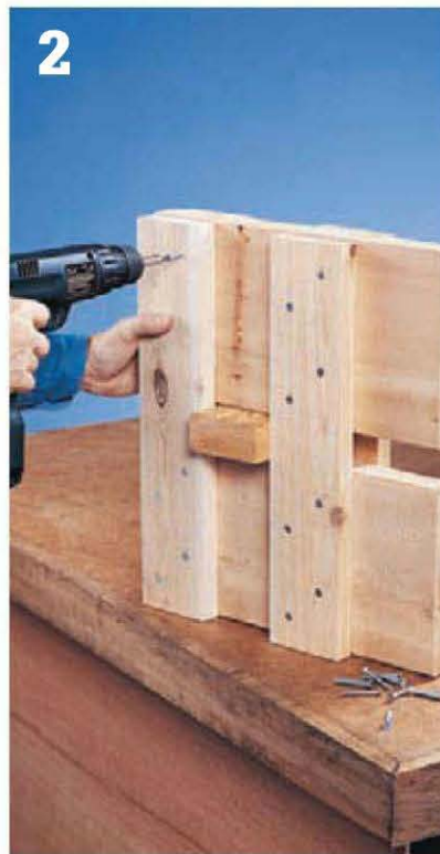
2 Attach the remaining leg half to the cleats on both ends, sandwiching the trestle on all sides.
