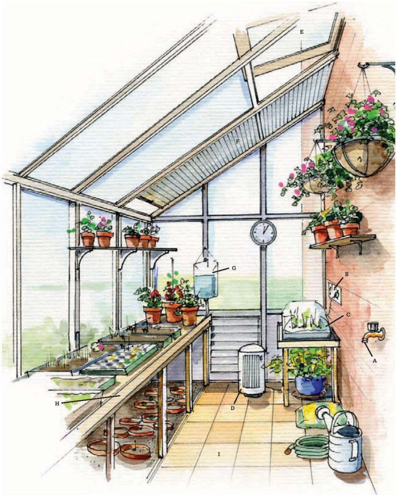
Attached to the exterior wall of the house, this lean-to style greenhouse has all the features for complete growing success: running water (A); electrical service (B); a heated plant-propagation table (C); a heater (D) for maintaining temperatures on cold nights; ventilating windows (E) and sunshades (F) for reducing temperatures on hot days; drip irrigation system (G) for maintaining potted plants; a full-length potting bench (H) with storage space beneath; paved flooring (I) to retain solar heat.
