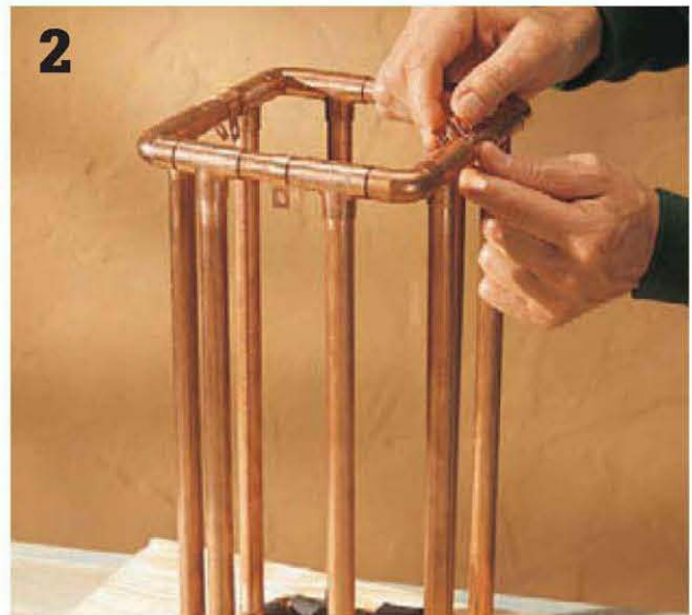
2 Bend pipe straps around the sides of the frame, positioning them to support the covers on the base and top of the lantern.
