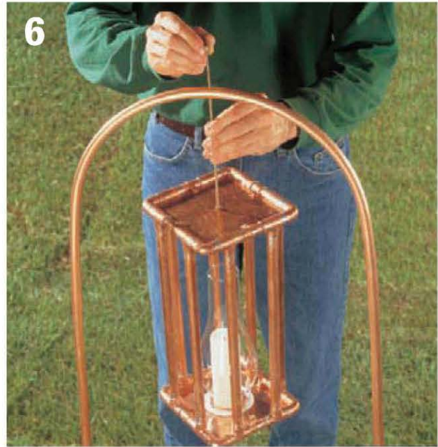
Add a nut to the top of the hanging rod; slide it through the hole in the supporting arch. Secure the rod with an acorn nut.
