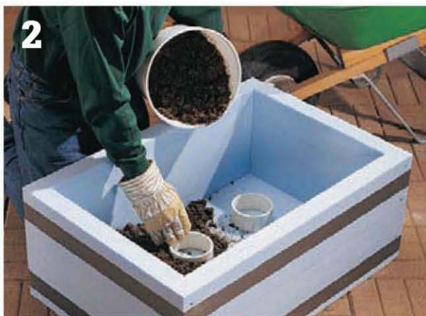
Pack hypertufa onto the floor of the form; press it down firmly to create a level, 2"-thick floor.
