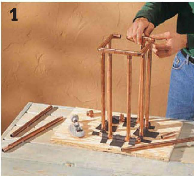
1 Connect copper pipes, elbows, and tees to form the base of the frame, and then add the legs and top.
