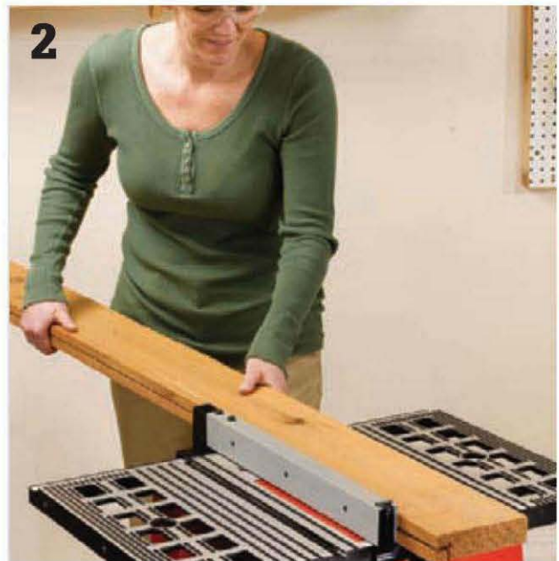
Cut panel rabbets. Make the 3/4 × 3/4" rabbet cuts in the rail stock using a table saw or router. The rabbets will accept the plywood side panels.
