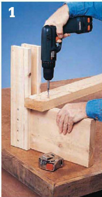
1 Attach the trestle to the legs, making sure it is positioned correctly against the top cleat bottoms.
