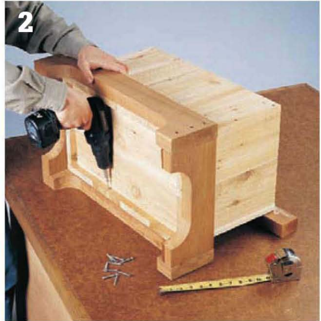
2 The recess beneath the bottom boards in the planter bin provides access for driving screws.
