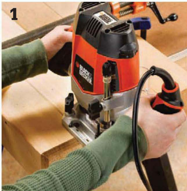
Make the posts. After cutting them to length from 4 × 4 cedar, make a 1/2" chamfer cut around all the tops. Gang the posts together for profiling if you like.
