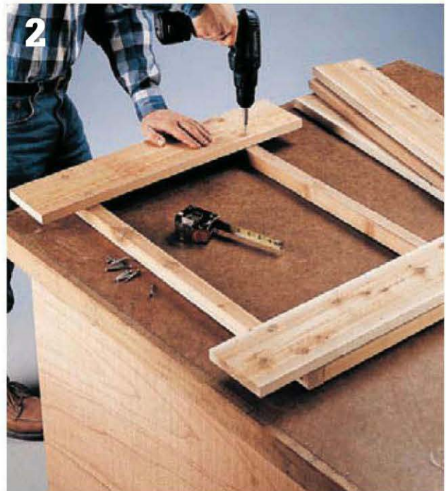
2 Attach a slat at each end of the panel frame so the outer edges of the slats are flush with the outer edges of the frame.
