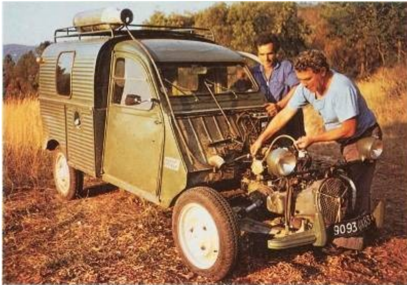
17 / 09 / 78 First motor vehicle to be run on BRUSHWOOD GAS.
