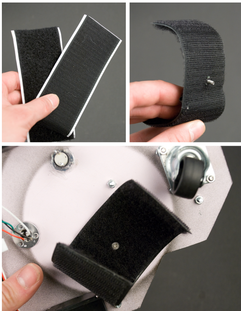
Figure 1-20. 14 cm strips of Velcro attached into the bottom of the chassis
