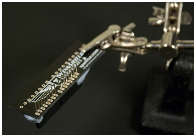
Figure A-3. Headers ready to be soldered
