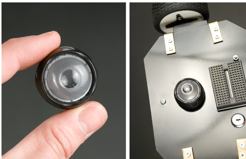
Figure 1-17. Lens glued on top of the chassis
