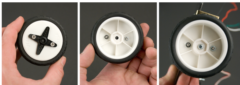
Figure 1-15. Servo horn attached to the tire rim and wheel attached to the servo
