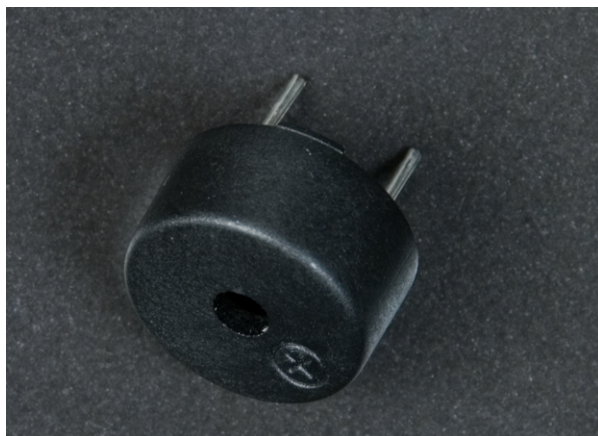
Figure 2-22. Small plus marks the positive leg of piezo speaker
