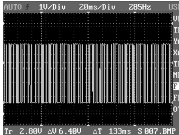
Figure 7-21. A 285 Hz PWM signal based on a 1200 stepsPerRevolution value
