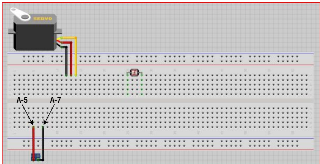
Figure 27-6. Attach the two-position terminal block to the breadboard
