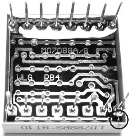
Figure 6-18: Pins on the LED matrix with a tiny 1 printed below the bottom-right pin
