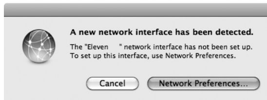
Figure 1-9: A new Arduino board is detected. Your dialog may read Uno instead of Eleven.
