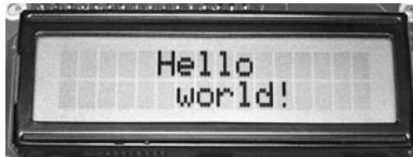
Figure 7-3: LCD demonstration: "Hello world!"
