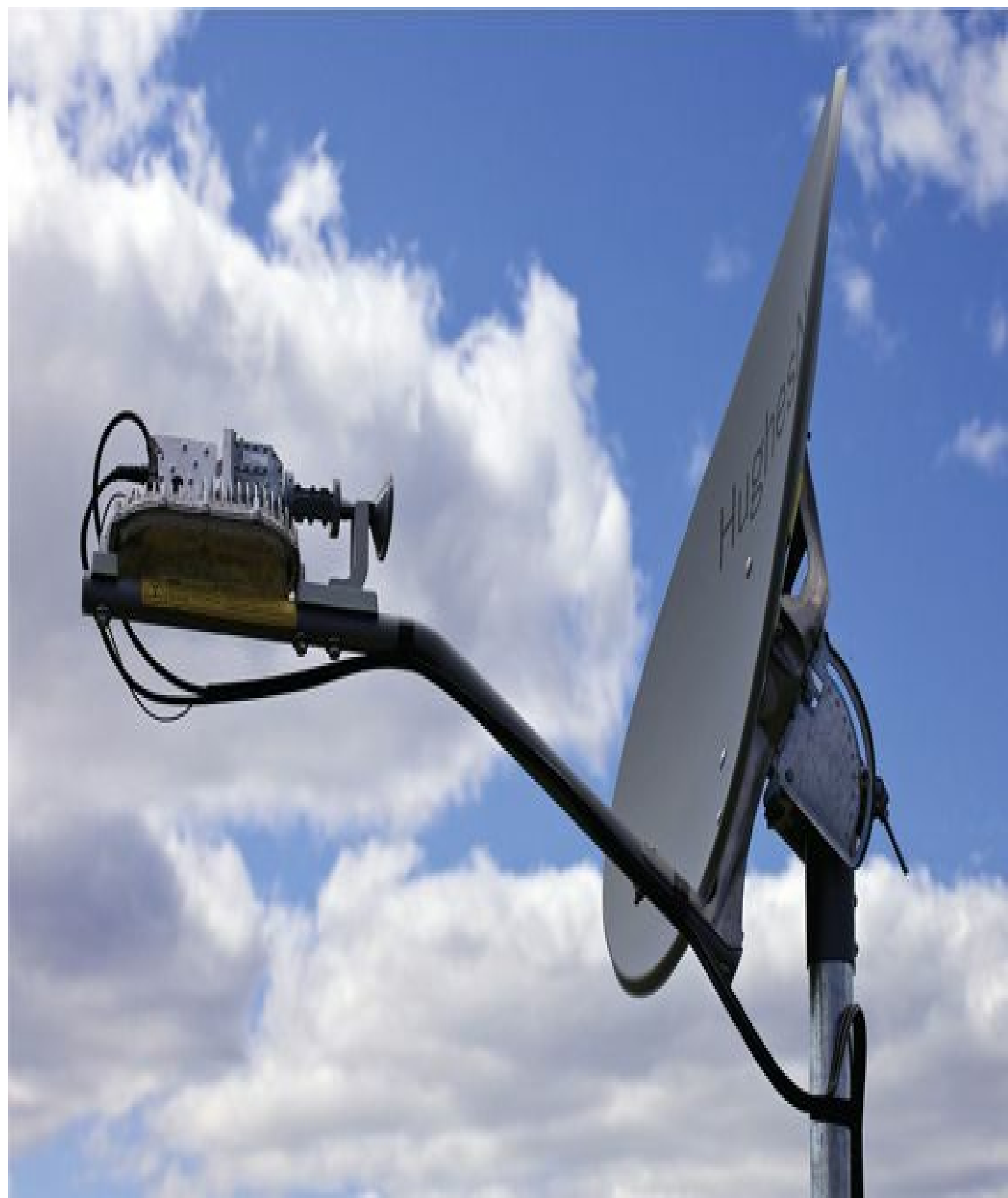
FIGURE 11-1 This satellite dish is stationary, yet it is always pointed precisely at a geocentric satellite.
