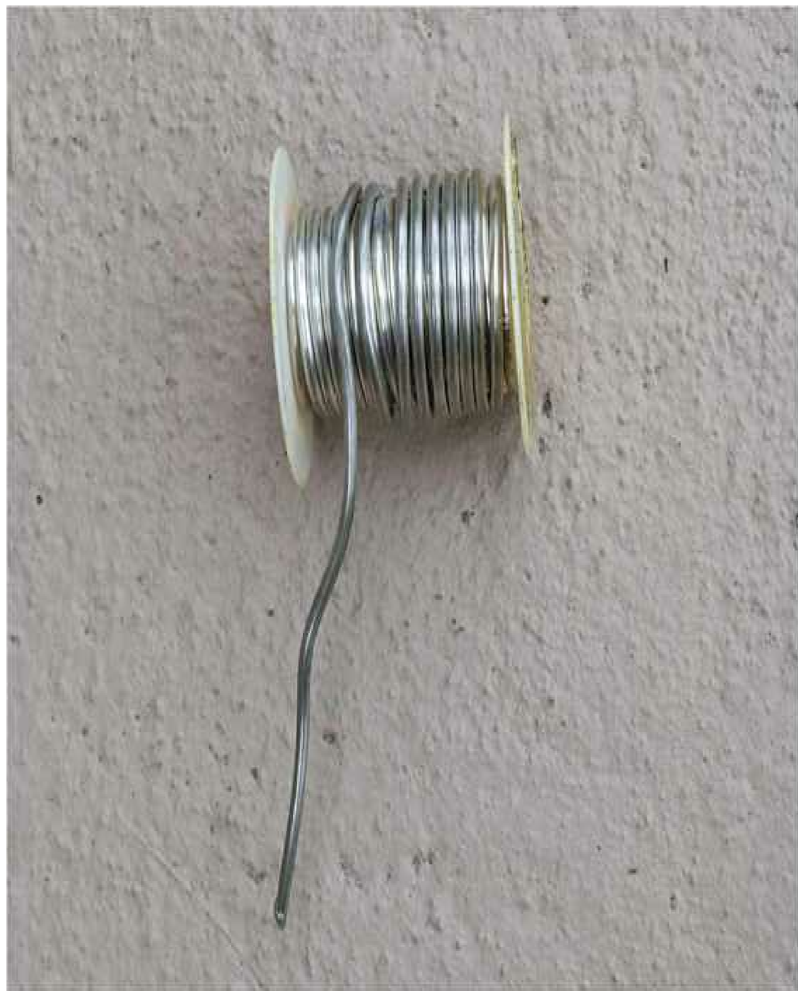
FIGURE 10-4 Wire solder for joining 12 American Wire Gauge (AWG) wire and larger.
