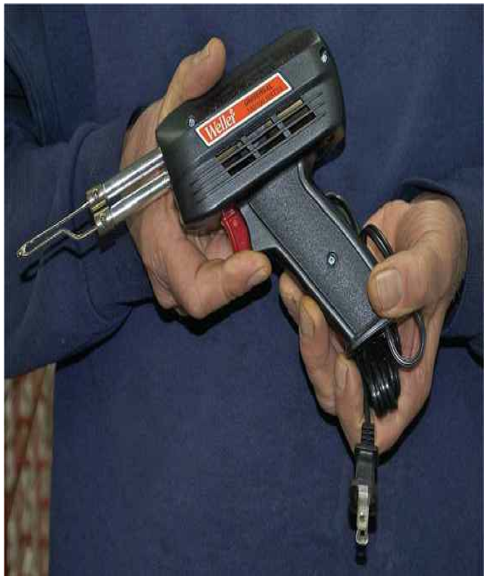
FIGURE 10-5 Pistol-grip soldering iron for large work.
