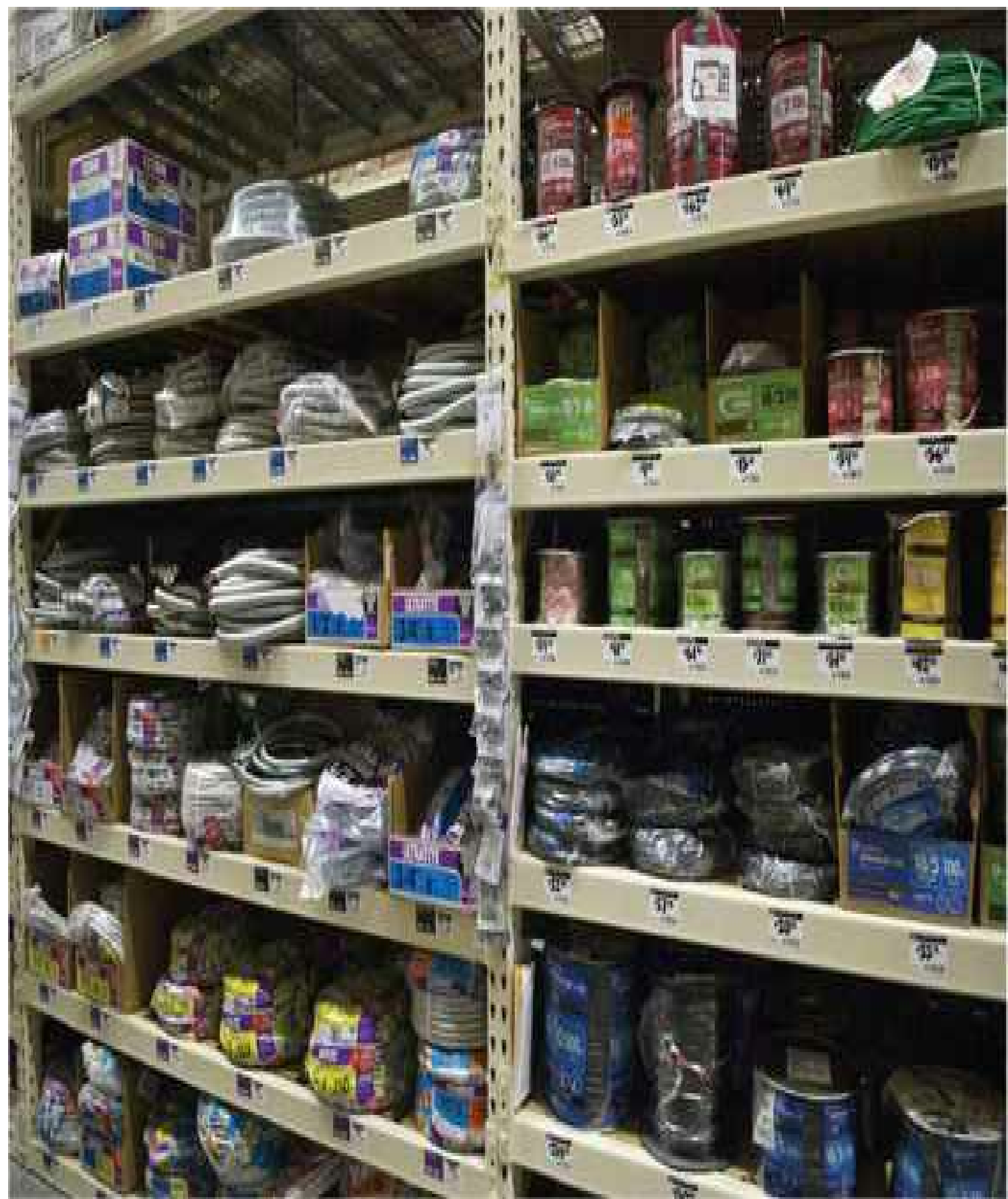
FIGURE 5-3 Type NM cable, at left, has many uses, such as powering a hot-water heater or submersible well pump for a home.
