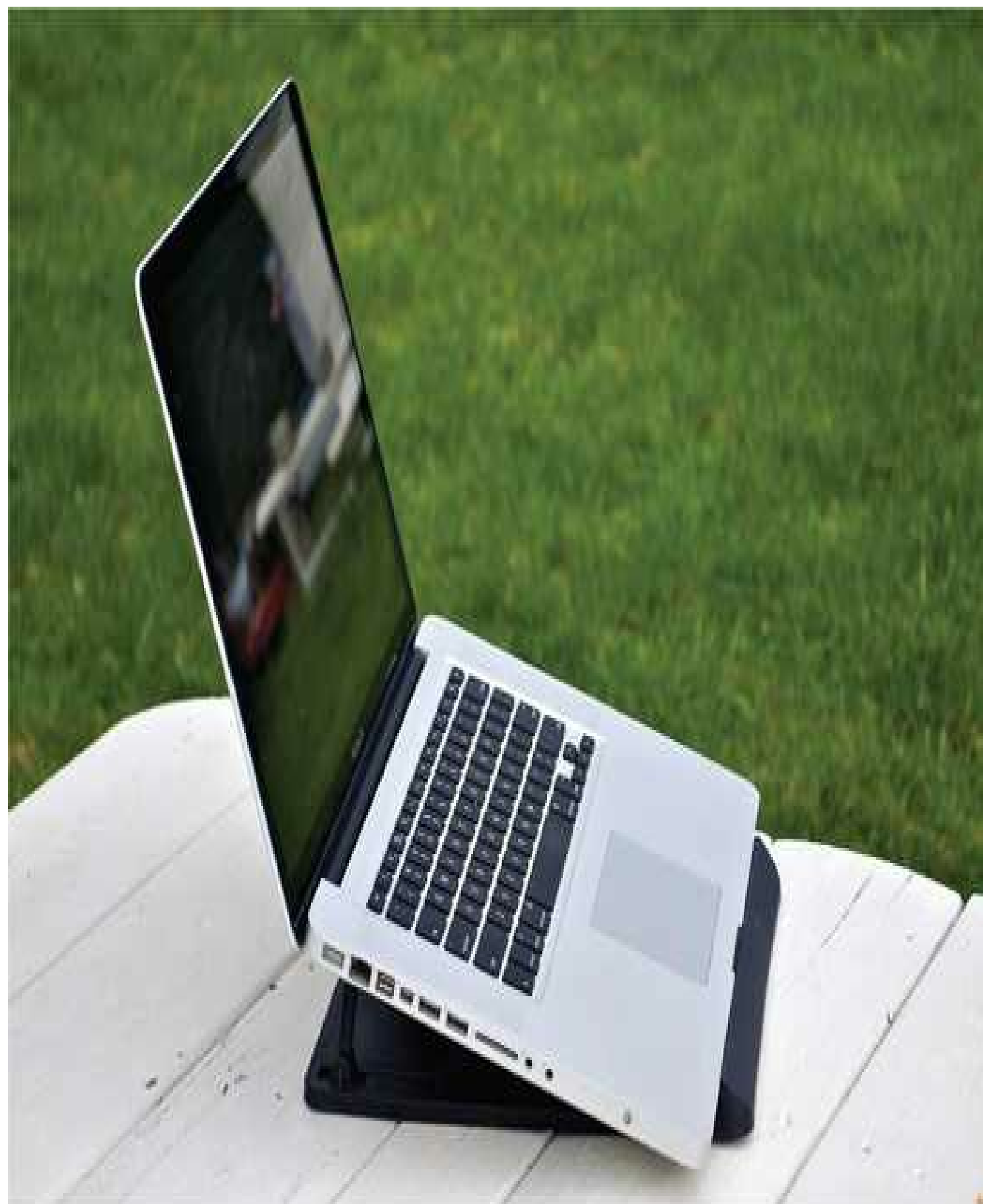
FIGURE 10-7 A stand improves air circulation and is highly recommended for long life of the laptop.
