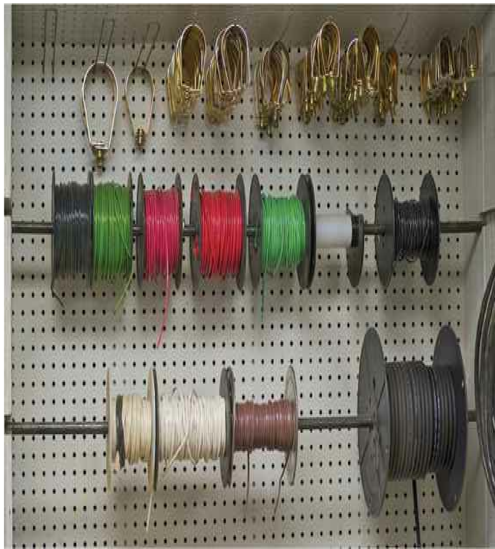
FIGURE G-4 Conductors are available in many colors, aiding in identification.
