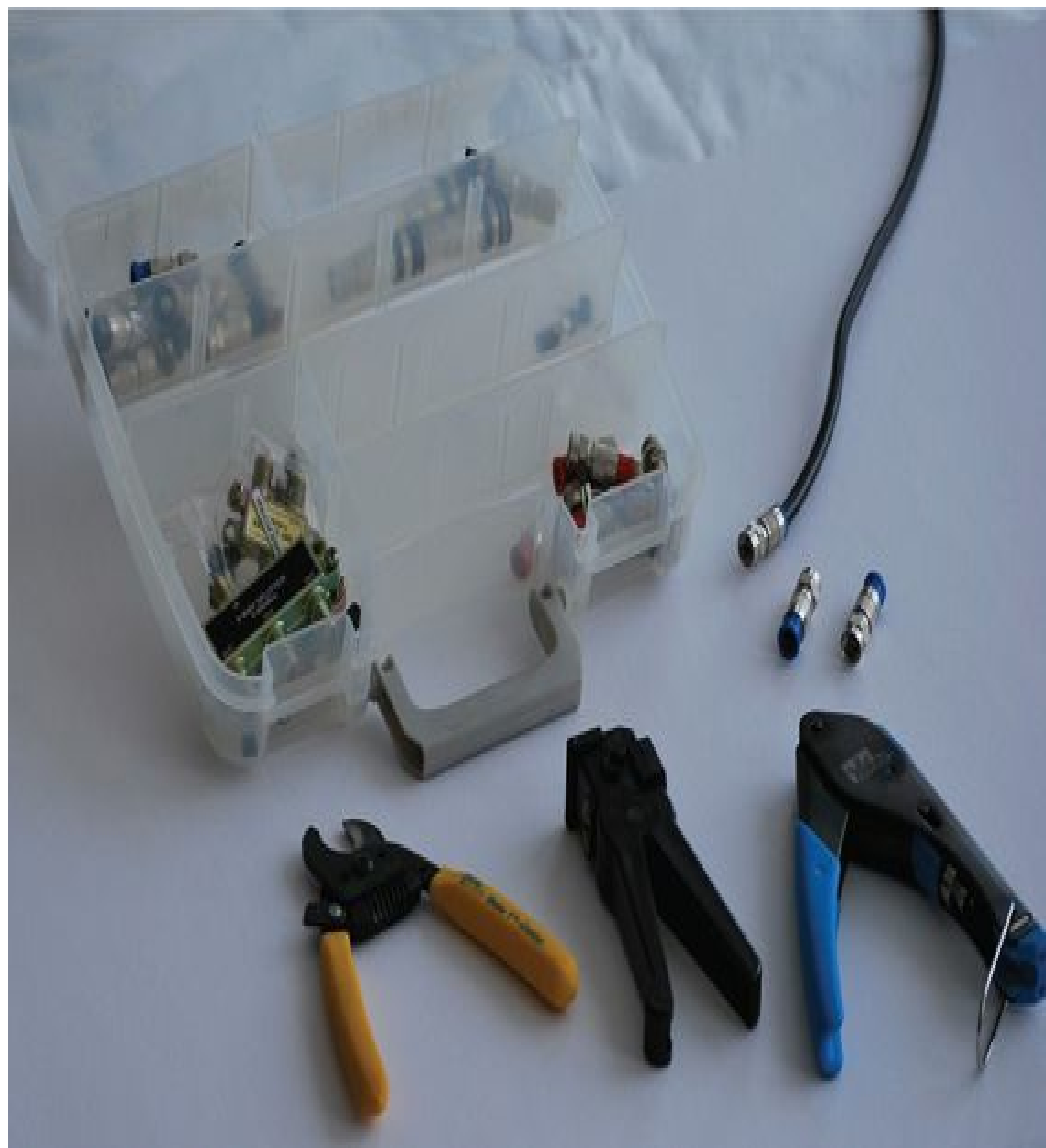
FIGURE 11-4 Coaxial cable with a connector, tools including a crimper, and an assortment of fittings.
