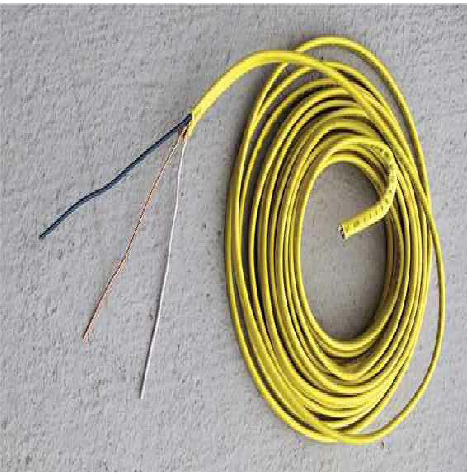
FIGURE 7-9 Romex cable is available in many colors, and using a selection of them is helpful in tracing branch circuits.
