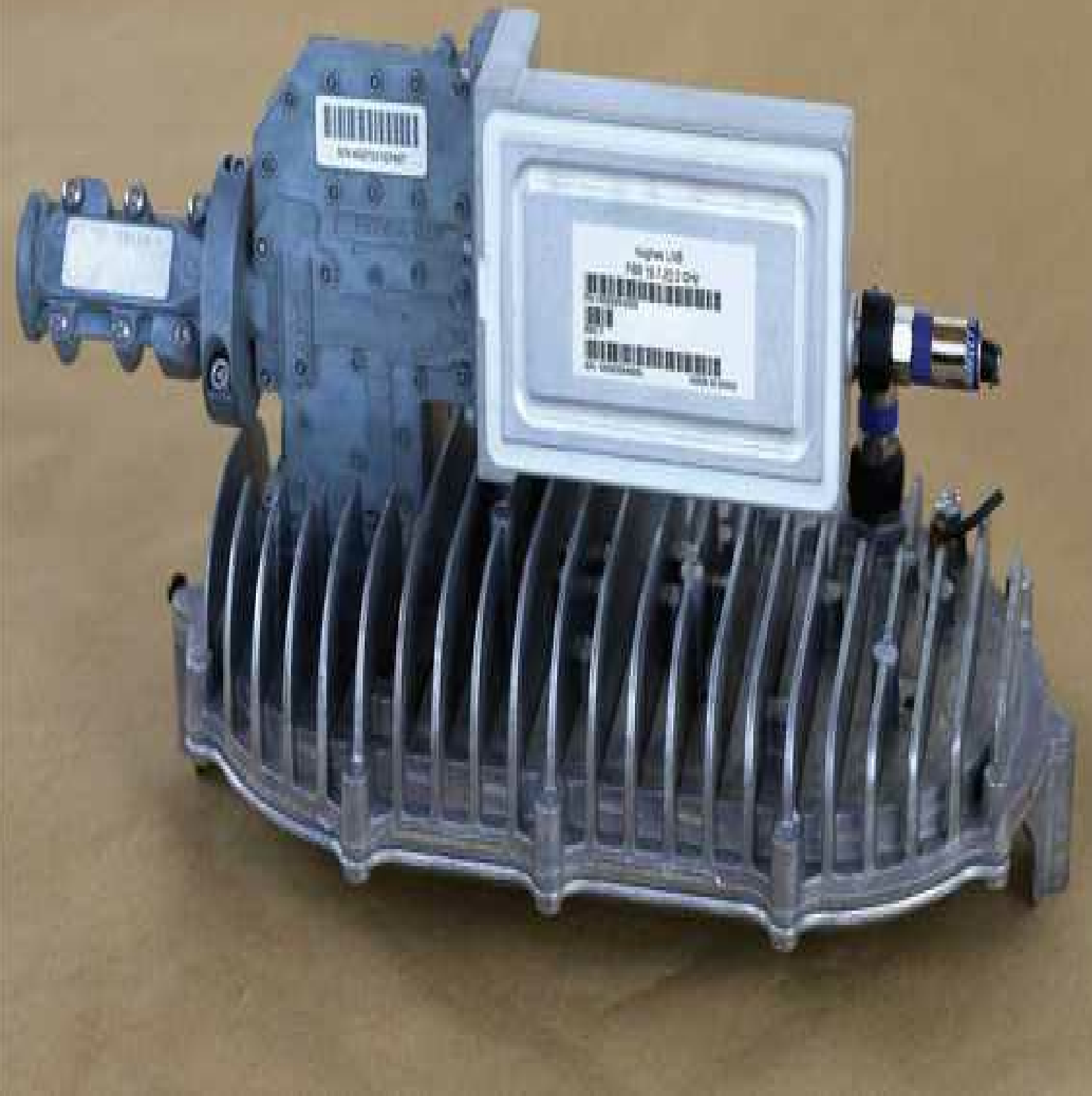
FIGURE 11-2 The low-noise block performs several functions associated with processing a satellite transmission.
