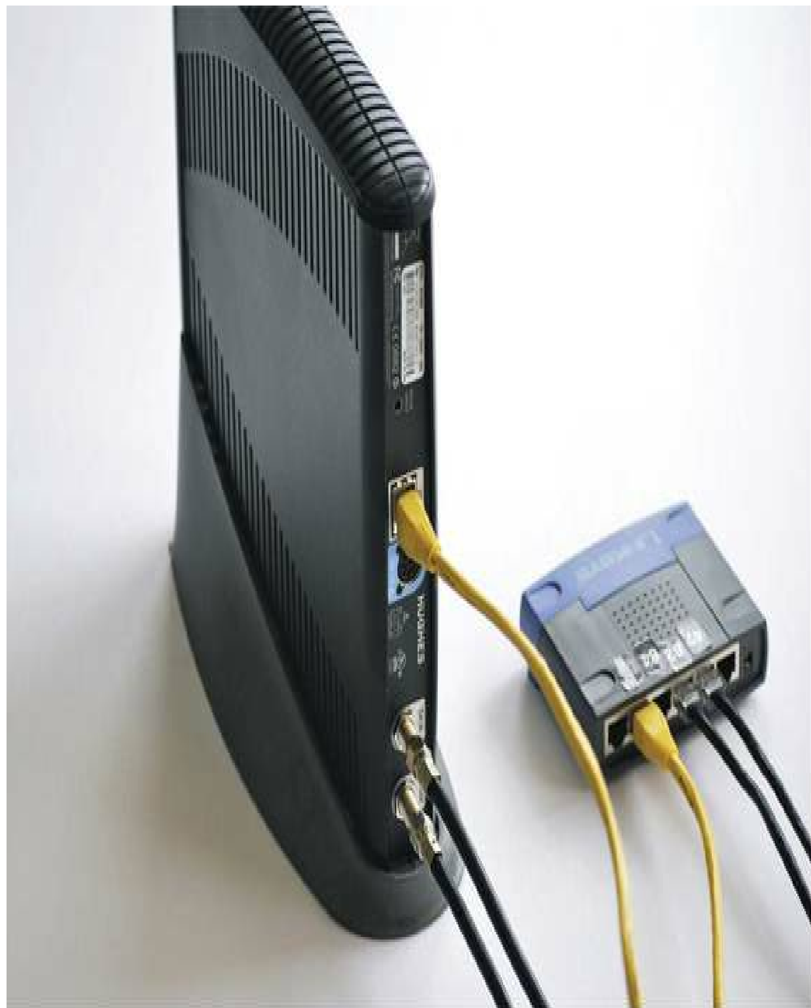
FIGURE 11-6 Modem for Internet access satellite dish system. Notice the two coaxial cables, one for
