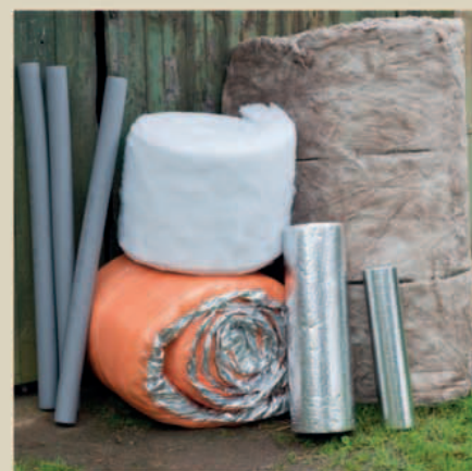
Insulation for every situation From left, expanded foam for pipework, recycled plastic fleece, a jacket for a hot water tank, foil reflectors for radiators, and a large roll of sheep's wool loft insulation.
