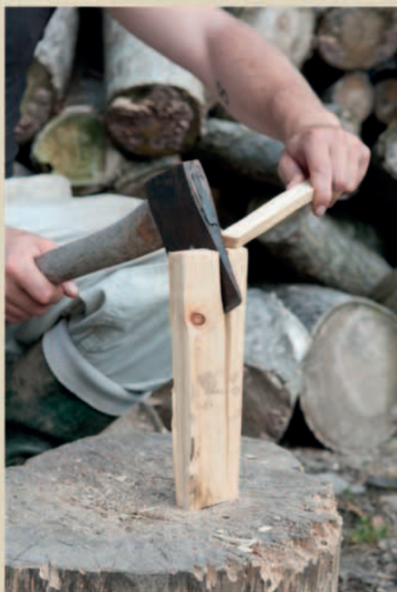
Never hold the wood you intend to chop; instead, hold it steady using another offcut while you cut into it with an axe.
