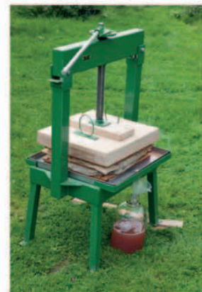
A screw press (34) for squeezing fruit to make wine, cider, and juices.
